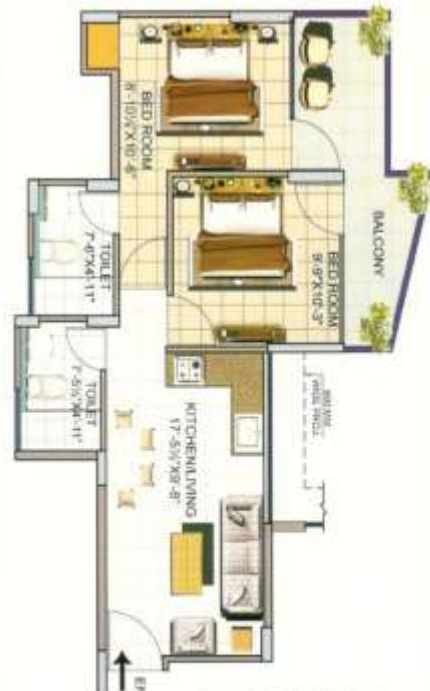
2 BHK UNIT PLAN TYPE-B CARRY AREA - 44.180 SQMT OR 475.514 SQFT BALCONY AREA - 5.175 SQMT OR 55.718 SQFT
